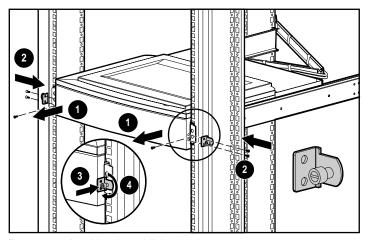
Figure 2-24. Attaching the stabilizing bracket
